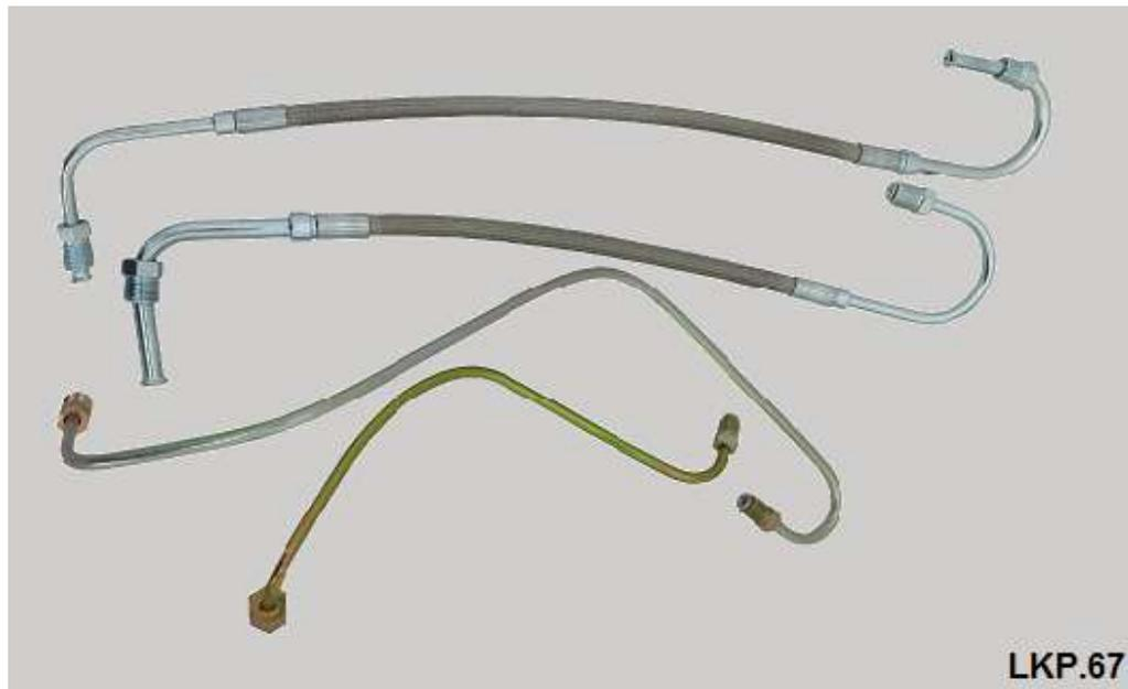
24. Connect the LKP.67 line kit as shown below. The images depict the installation of the under hood brake line kit components.
