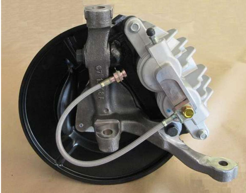
22. Fit a brake hose with a copper crush washers, 1 on the top and 1 on the bottom of the banjo fitting (fitting at caliper end of the brake hose). The brake hose set are identical, left and right.
