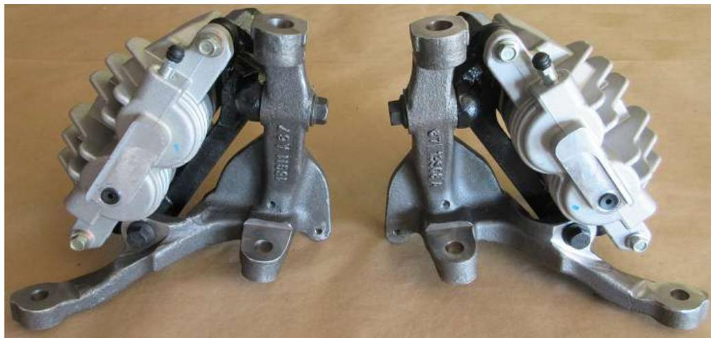
18. The caliper set are pre-assembled on their bracket, with all hardware and brake pads, ready for mounting over the rotor.
