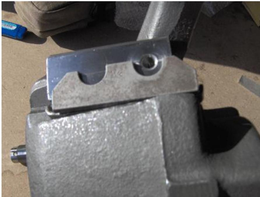
29. The key is properly positioned when the caliper retainer bolt can nest into the circular recess in the key.
