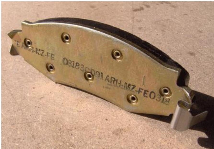
23. Turn the steering wheel to provide access to the inside of the caliper bracket. Insert the inner pad into its place, anti-rattle clip end first on the rearward end of the bracket. Press the friction surface against the rotor. See the photo below for a guide to the pad orientation. The anti-rattle clip is located at the left side in the photo. THE CLIP AND PAD WILL FIT, BE PERSISTANT!
