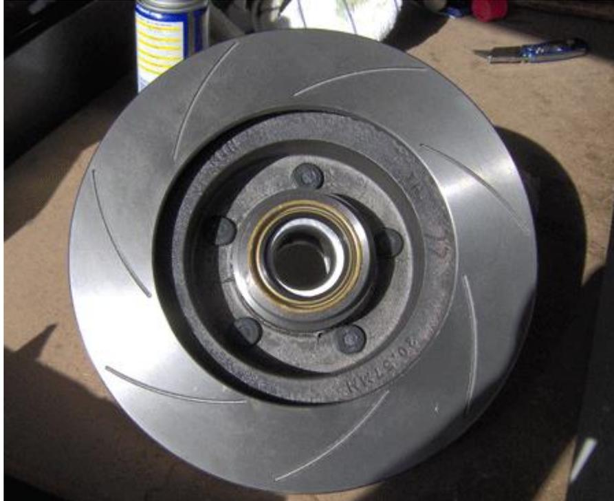
5. Apply a scant amount of grease to the wheel seal's sealing surface on the spindle. Carefully insert the rotor onto the spindle. Don't scrape the seal over the threads on the end of the spindle. You should be able to feel the seal slip over the sealing surface on the spindle.
