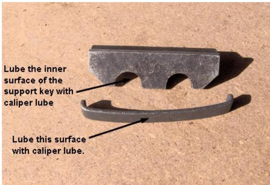
28. Using at least two hands and a foot, hold the caliper in place and insert a support key-support key spring assembly. Use a hammer (and one of your other hands) to drive the support key assembly into place between the bracket rail and the caliper keyway. The key will seat very tightly. This is correct. See the photos below.
