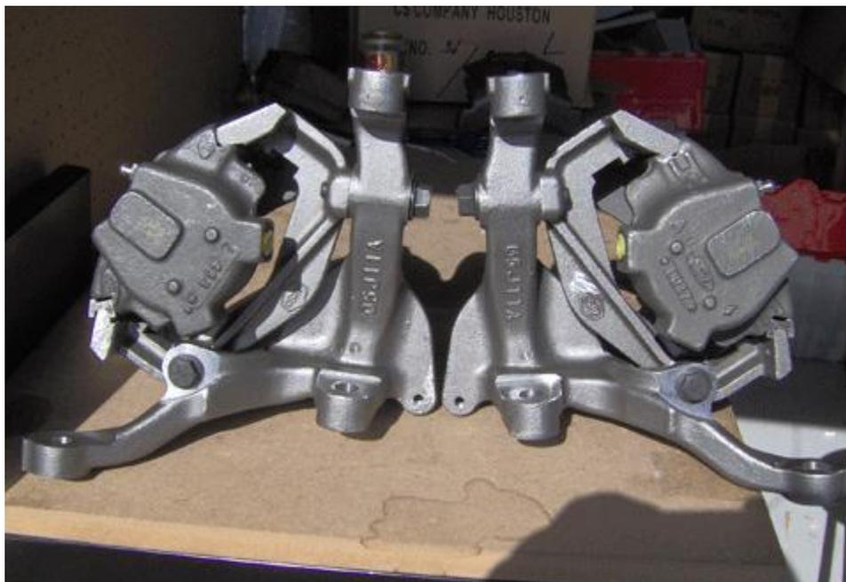
25. Place the outer pad into its place on the front inside of the caliper. Notice the tabs, on the pad, that wrap around the protrusion in the caliper. The
