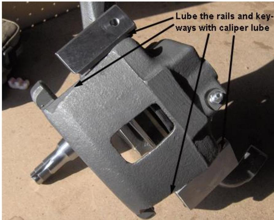
27. Apply a thin coating of caliper lube to the inner surface of the support key and the outer surface of the support key spring.
