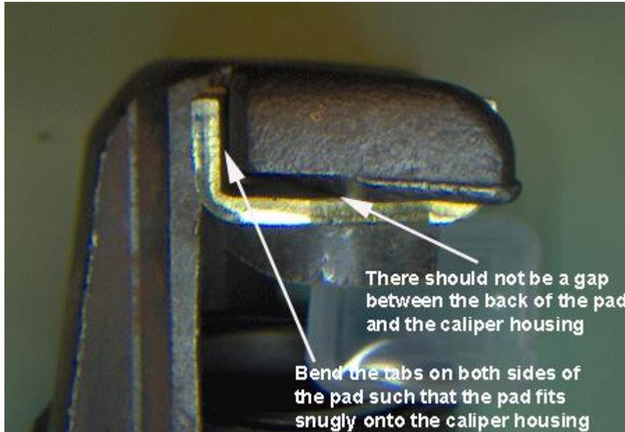
26. Apply a thin coating of brake caliper lube to the bracket rails and the caliper keyways. Slip the caliper onto its bracket. Insure that the rails on the bracket seat onto the keyways on the caliper and the brake pads are correctly positioned on each side of the rotor.
