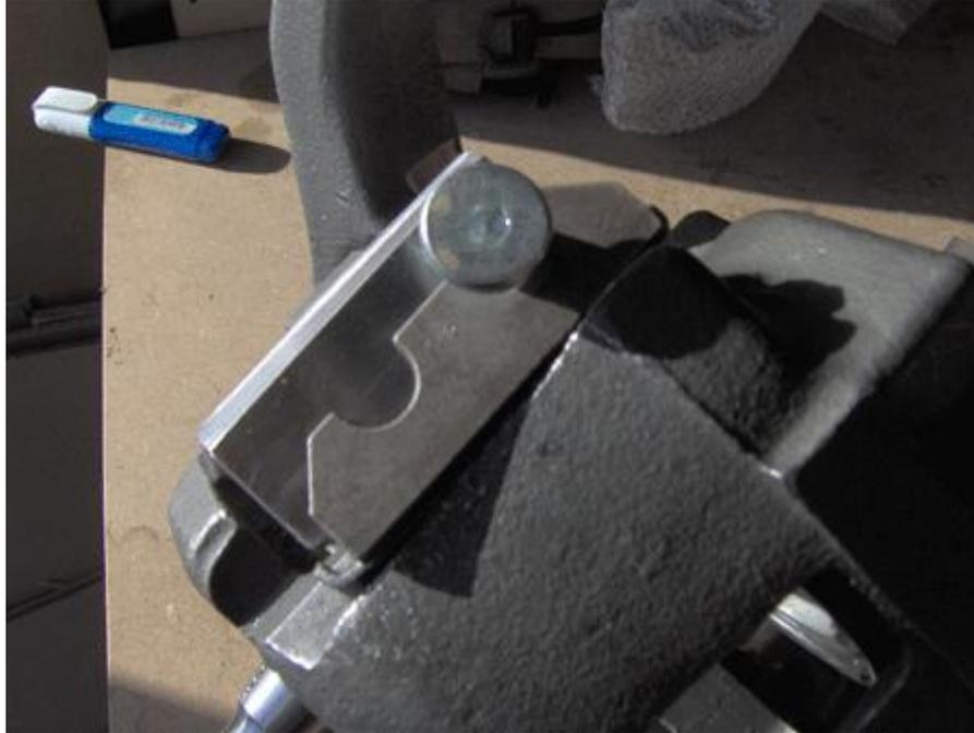
30. Thread the caliper retainer bolt into the bracket and torque it to 12-16 ft-lb. Thread locker has been pre-applied to this bolt.
